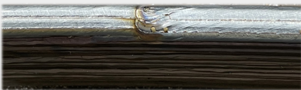
Close-up of overlap region from multi-robot WAAM system.
