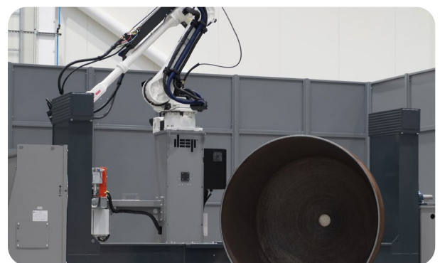
Production of Hemisphere's using DEEP Manufacturing Two Axis Manipulator Table.
